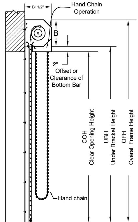
COIL SIDE ELEVATION
