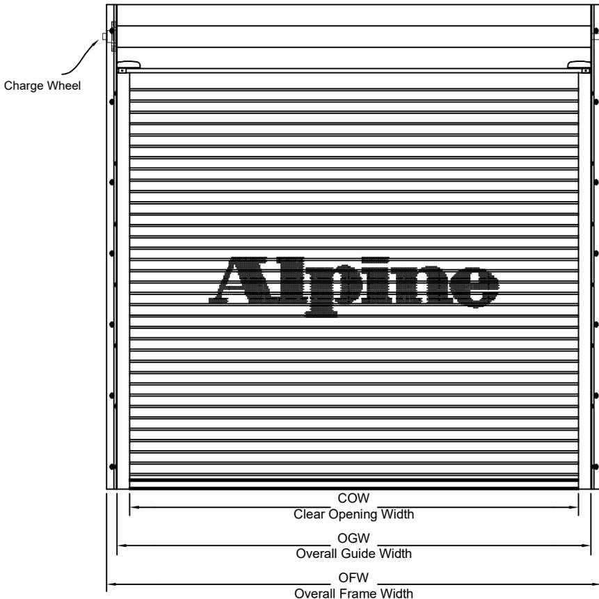
**COIL SIDE ELEVATION**
