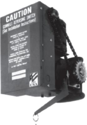
UL listed. High starting torque motor: removable without affecting the limit switch settings. Full overload protection. Low voltage control circuit, 24 VAC. Factory pre-wired all electrical components in a NEMA 1 enclosure. Dual relay system with a 3 button, NEMA 1 control station included. For use on small rolling grilles and counter shutters where manual chain hoist is not required. Heavy duty #41 roller chain and drive sprocket enhances the final drive.
